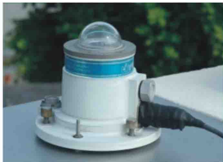
Instrument for measuring UV Index by the Observatory at King's Park
