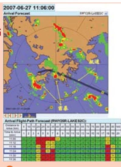
Figure 2: Prototype of one of the aviation specific weather products which gives short-term prediction on thunderstorm activities in Hong Kong and the surrounding air space
