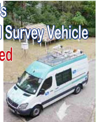
▲ The new radiological survey vehicle, with new meteorological instruments installed on its top, can collect both radiation monitoring data and weather information at the same time.
