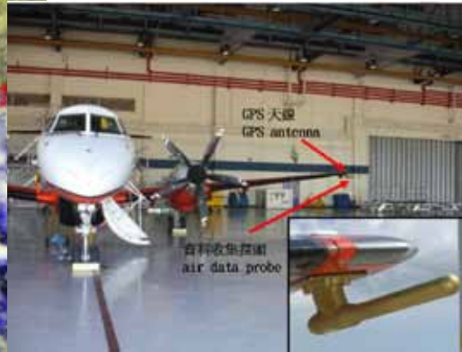
▲ The meteorological measuring system installed on the fixed-wing aircraft, with the inset showing the air data probe.
