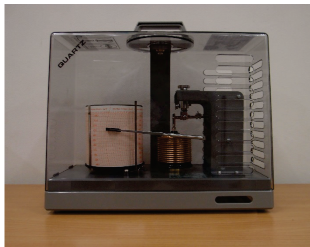
Figure 3 - A barograph for continuous recording of atmospheric pressure.
