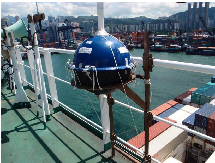
Figure 1. An automatic weather station installed on board a HKVOS
