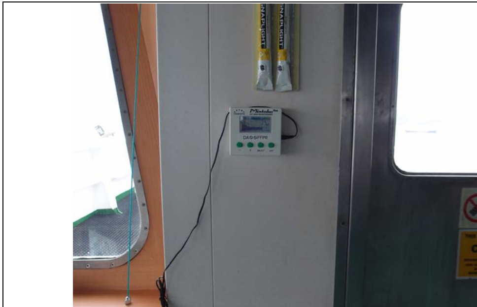
Figure 5. First digital barometer installed on board Hong Kong VOS Dapeng Moon in 2016
