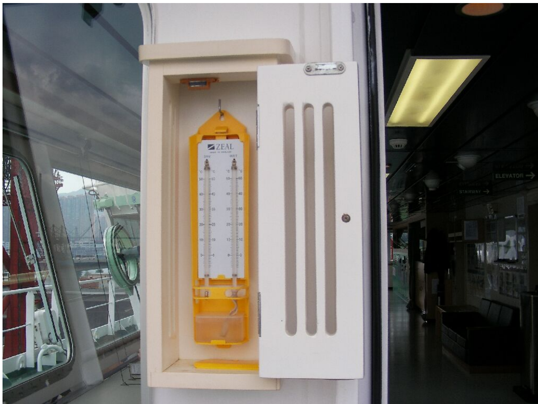
A hygrometer and shelter installed on HKVOS
