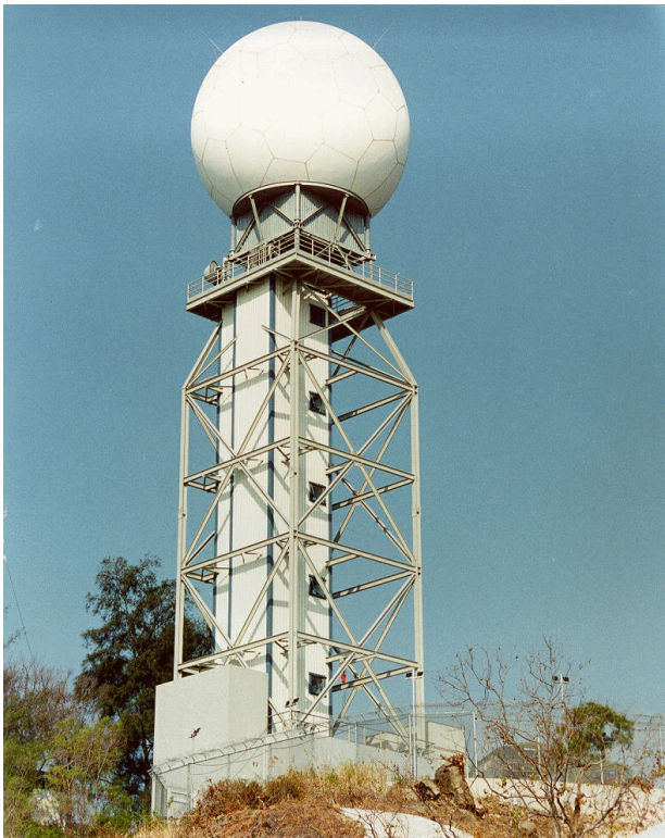
Weather sensors for monitoring wind shear and turbulence conditions in and around Hong Kong International Airport include a terminal Doppler weather radar.
